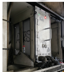
Buck Inverter mounted on monorail
