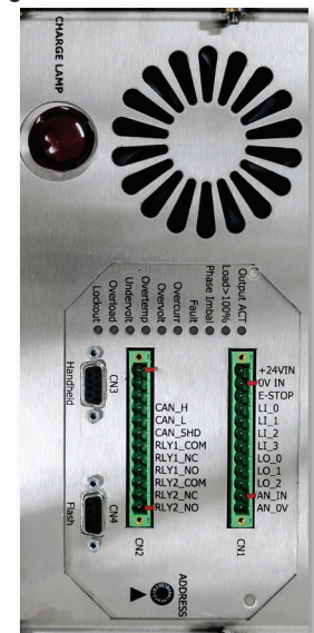
Top panel with fan exhaust, indicator lights and I/O connections
