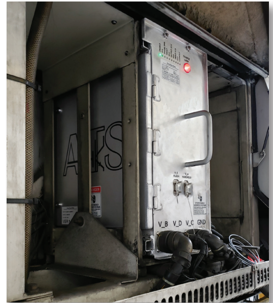
Example of Buck Inverter installed on light rail vehicle.
