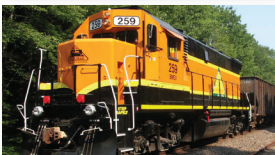
2009 Brookville Co-Gen Locomotives 1.5 MW DC Propulsion Systems
