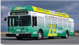
1997 (as Saminco International) Ballard / XCELLSIS Phase 1-5 Bus Program Hydrogen Fuel Cell Bus 650V DC 350kW VFD system
