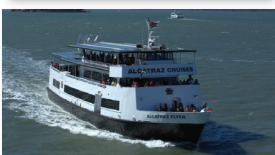
2012 Alcatraz Clipper Passenger Ferry Dual 700 kW AC Propulsion Hybrid System Battery Chargers Auxiliary Power Supplies
