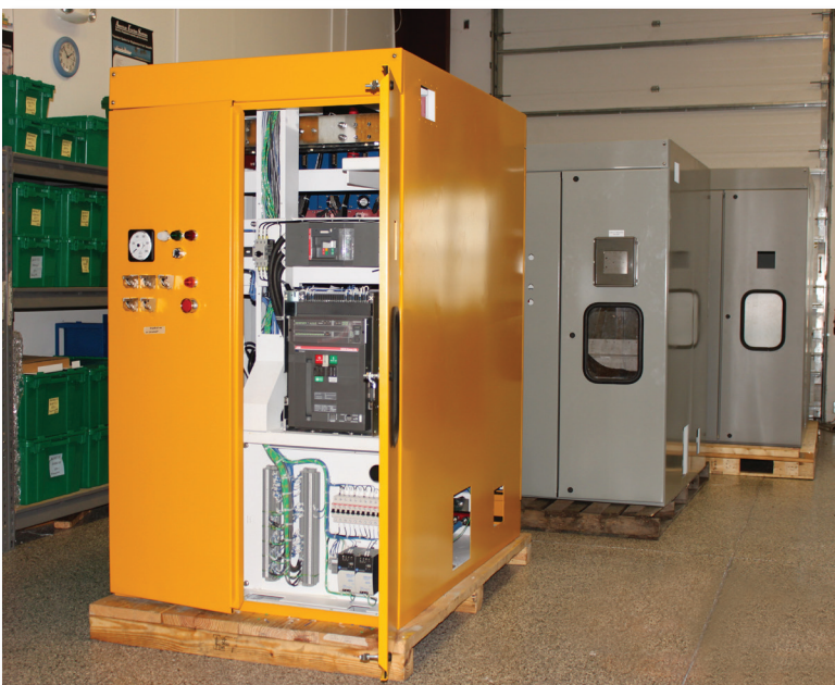
AC and DC Locomotive Traction Lockers
