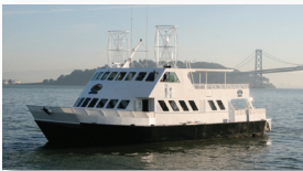
2008 Alcatraz Hybrid Passenger Ferry Dual 300 kW AC Propulsion Hybrid System 1st North American Hybrid Passenger Ferry
