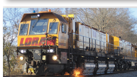
2021 Loram RGS Series MoW Grinder, Australia AC Traction System for Dual AC motors
