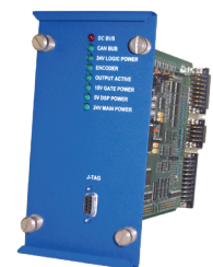
ATS Control Card Assembly
