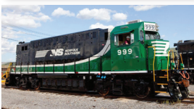
2010 Norfolk Southern 999 Locomotive 500 kW DC Propulsion Battery System
